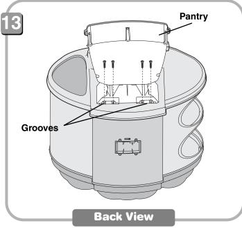
Insert four screws through the grooves in the pantry and into the counter top. Tighten the screws with a Phillips screwdriver. Do not over-tighten.
